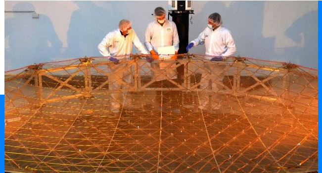
5 m large deployable reflector surface with HPtexas-USM-mesh under RF testing at Airbus Germany
